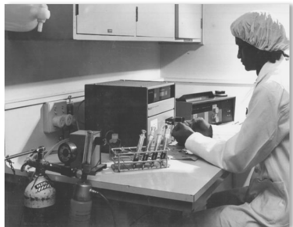
Jagdish (Jack) Bhana doing oximetry for cardiac output calculation using the OSM2, the older haemoreflector alongside (above right).
